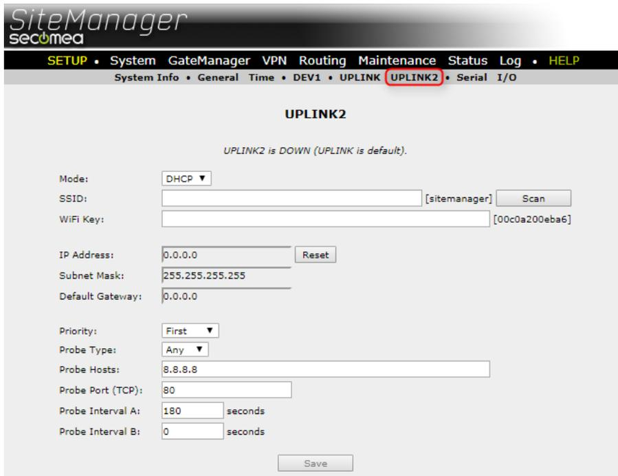
The screenshot shows the SiteManager web interface for the UPLINK2 configuration page. The breadcrumb trail is: System Info • General Time • DEV1 • UPLINK • UPLINK2 • Serial I/O. The page title is UPLINK2. A message states: UPLINK2 is DOWN (UPLINK is default). The configuration fields are as follows:
