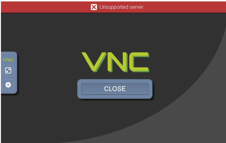
The message “Unsupported server” was observed on units like a Siemens TP277 panel with SmartServer/VNC server installed.
