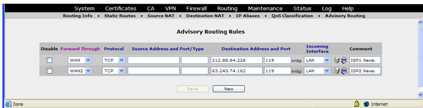
Figure 6 Traffic from each ‘NEWS provider is directed to a different WAN interface
